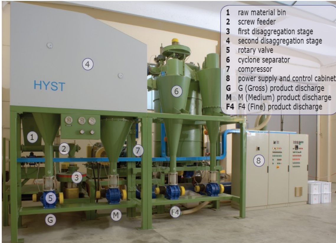
HYST system for the energy sector (working capacity: 1-5 t/h)
